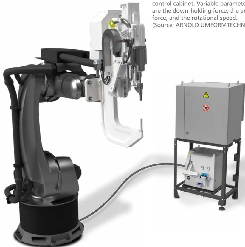
Picture 4: The system consists of a feeder unit, a joining unit and the control cabinet. Variable parameters are the down-holding force, the axial force, and the rotational speed. (Source: ARNOLD UMFORMTECHNIK)
