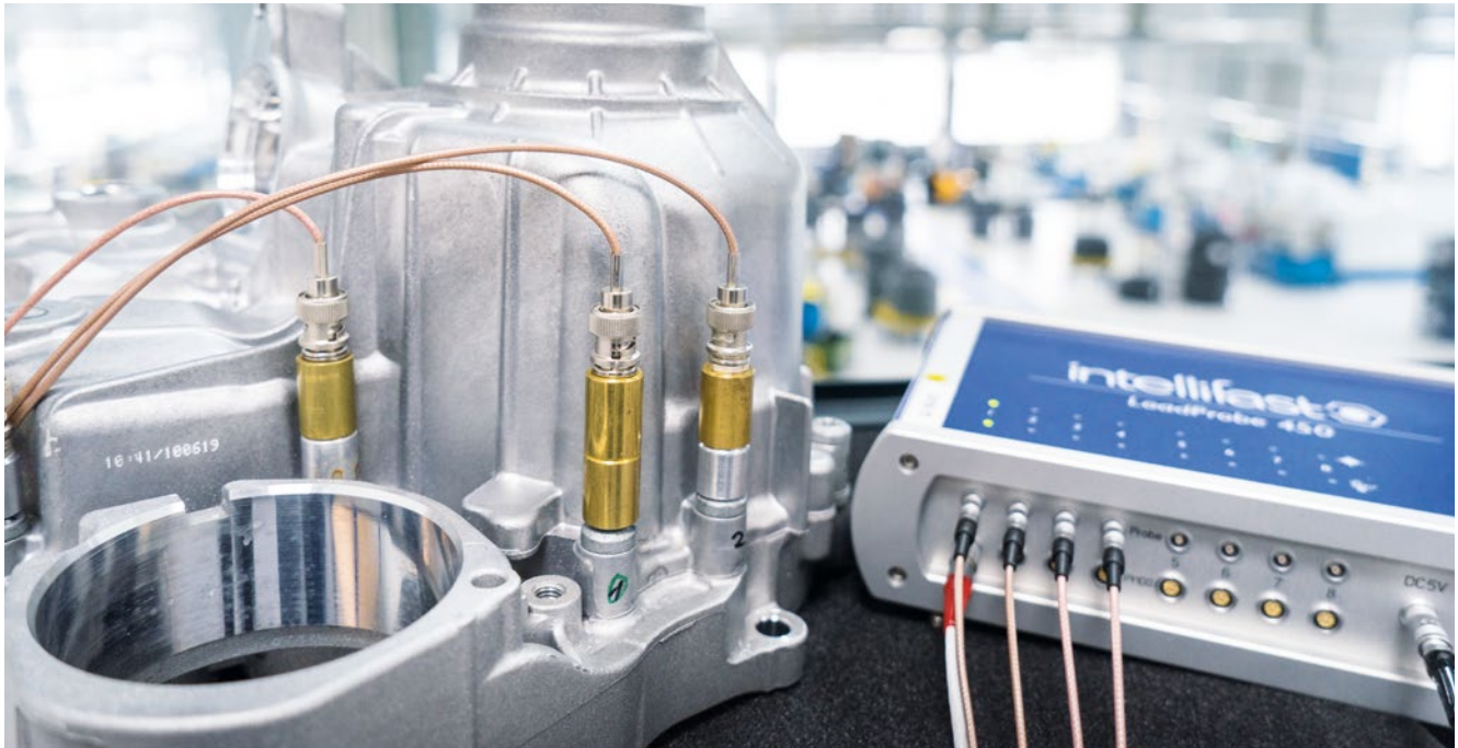
Picture 2: Clamp loads in the original application are determined using ultrasound measurement technology. (Picture: ARNOLD UMFORMTECHNIK)
