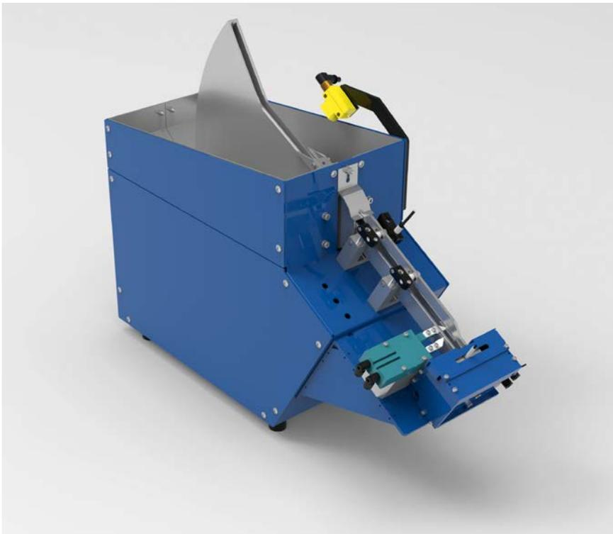
Figure 1: Basic structure of the sword feeder. The upward and downward movement of the sword feeder sorts the screws into the correct position and conveys them to the conveyor unit's buffer area. They are separated here and compressed air then moves them onward to the processing unit. (Source: ARNOLD UMFORMTECHNIK)
