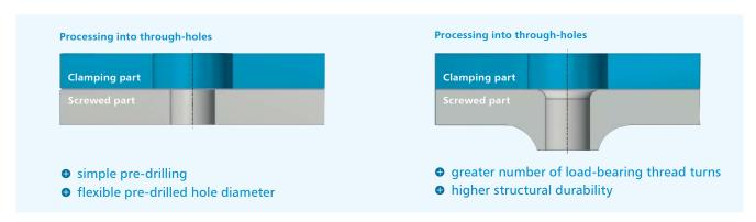
The anticipated process and assembly parameters can be optimally adapted to the application in question due to the flexible dimensioning of the pre-hole diameter in the screwed part.
