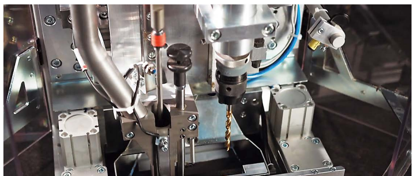
Picture 3: The ASA's integral process monitoring makes it possible to control the drilling and screwdriving processes. In addition, faulty operations are detected quickly and can be corrected promptly.
